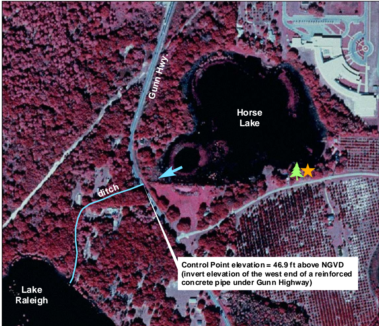
Figure 2. Location of lake water level gauge, hydrologic indicators, outlet, control point, and outlet conveyance system for Horse Lake.
